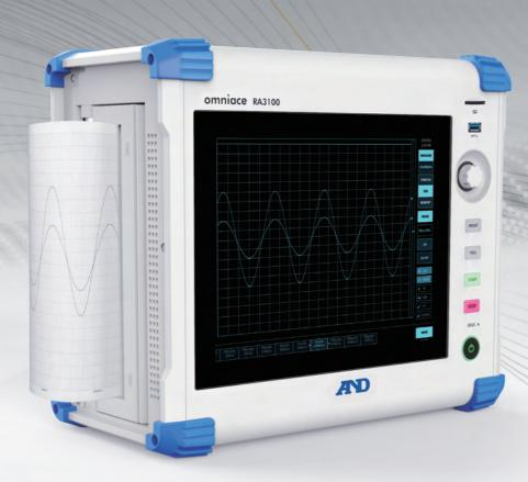
Omniace RA3100 is a data acquisition system for research, development, and field maintenance, which enables accurate and long-term measurement of high-speed switching waveforms, even in severely noisy environments, in electric automobiles, electronic appliances, railroad cars, and solar power generation systems utilizing inverter control technology that has become widespread in recent years.
