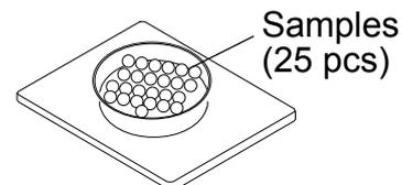
6. Press the **ENTER** key to calculate and store the unit weight. Remove the sample.
