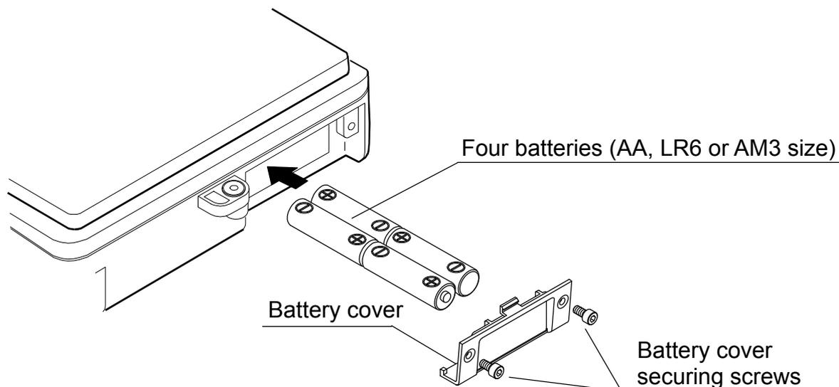
4. Attach the battery cover and secure it to the balance using the battery cover securing screws.
