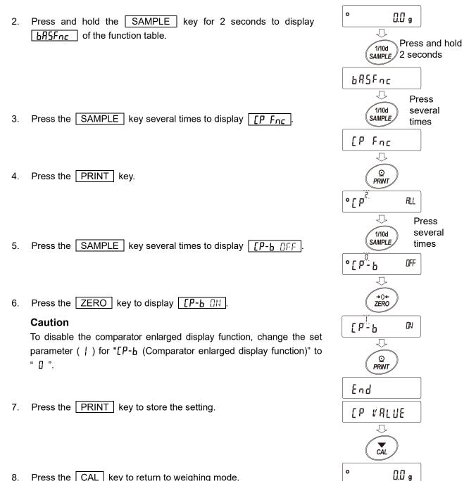
Press the CAL key to return to weighing mode. 8.
