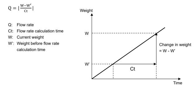
The FRD function stores the weighing data in the balance and calculates the flow rate.
