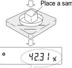
Note The stored 100% reference mass is stored in nonvolatile memory even if the power is removed.
