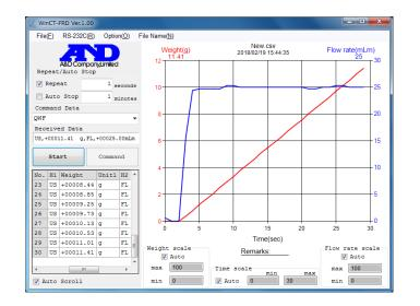
□ Weighing and flow rate data can be simultaneously output to an external device.
