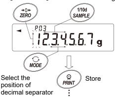
2. To use the newly stored unit weight, press the **PRINT** key to select the value. The balance returns to weighing mode.
