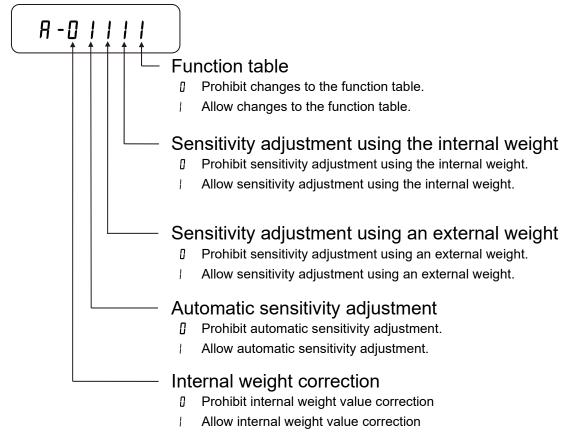
Example: Function selection switches of GF-L series (display at factory settings)
