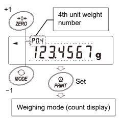
3. Press the **PRINT** key to set the unit weight to use. The balance returns to weighing mode (count display).
