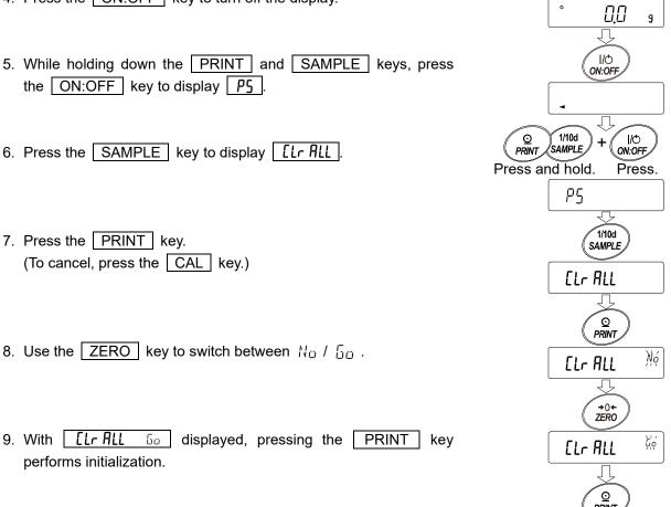
10. When initialization is completed, the balance automatically returns to weighing mode.
