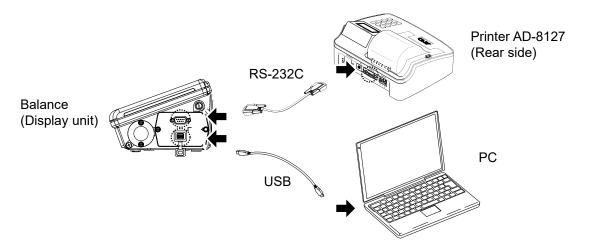
If only the balance is connected to the PC, it can also be connected using a USB cable or RS-232C cable.
