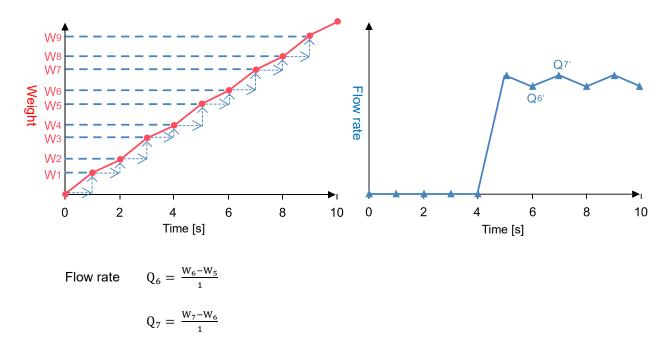
In this example the 1 second change in weight is the flow rate value. Therefore, when the weighing value varies greatly, the flow rate value also fluctuates. When the flow rate calculation time is 5 seconds:
