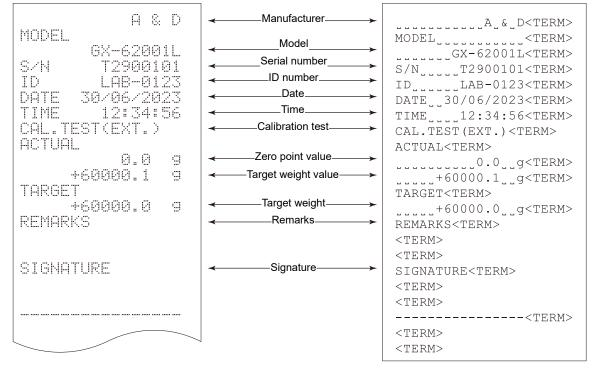
\_ : Space, ASCII 20h <TERM> : Terminator, CR LF or CR CR: Carriage return, ASCII 0Dh LF: Line feed, ASCII 0Ah
