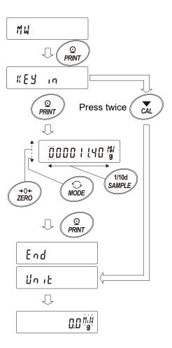
[Input using repeatability with an external weight]
