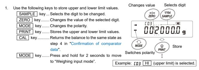
2. To use the newly stored comparator value, press the **PRINT** key to select the value. The balance returns to weighing mode.
