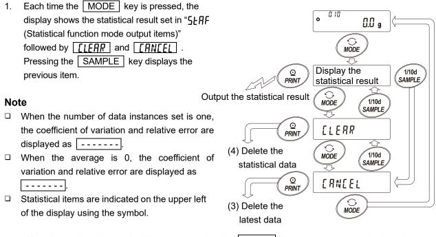
2. When the statistical result is displayed, pressing the **PRINT** key outputs the statistical result.
