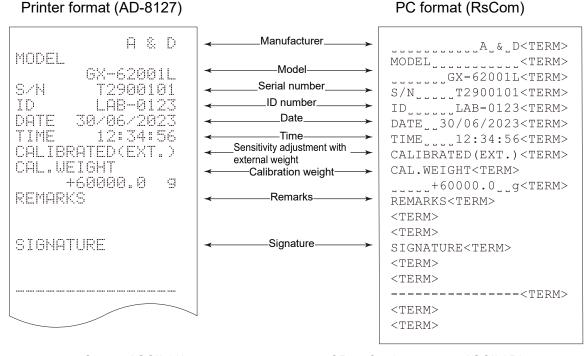
□ : Space, ASCII 20h <TERM> : Terminator, CR LF or CR CR: Carriage return, ASCII 0Dh
