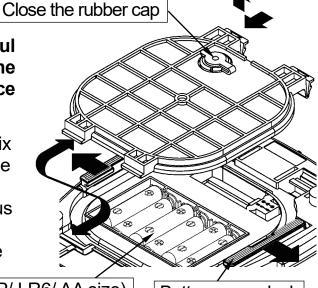
New six batteries (R6P/ LR6/ AA size)
