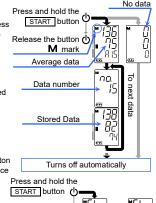
Release the YE 5 button no d Select "CL - YES" to clear data. The M mark blinks Data is cleared. Turns off automatically
