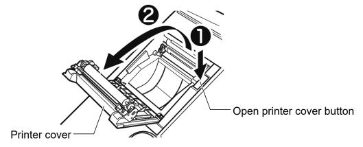
2. Install the printer paper in the way shown in the illustration below.
