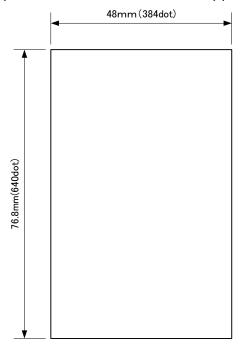
Create the bitmap data of the abovementioned size with a file name "Logo.bmp" and save it in the root folder of the SD card.
