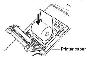
6. With the end of the paper at the top and protruding out, secure the printer paper by closing the printer cover until you hear a click. If the cover is not completely closed, a paper jam may occur.
