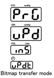
3. Insert the SD card containing the bitmap file (Logo.bmp) saved in "15.1. Size of original bitmap patterns" into the SD socket. Press the **START/STOP** button to start data transfer.
