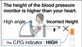
The position of the device is checked both before and after measurement If both checks show a correct measurement position the LEVEL indicator is lit(blue). For all other measurements an indicator for LOW or HIGH measurement position will be lit (orange).
