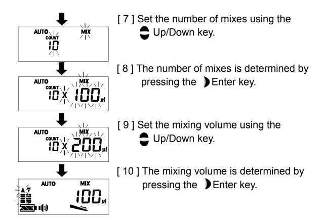
2) Operation method for Dispensing and mixing mode
