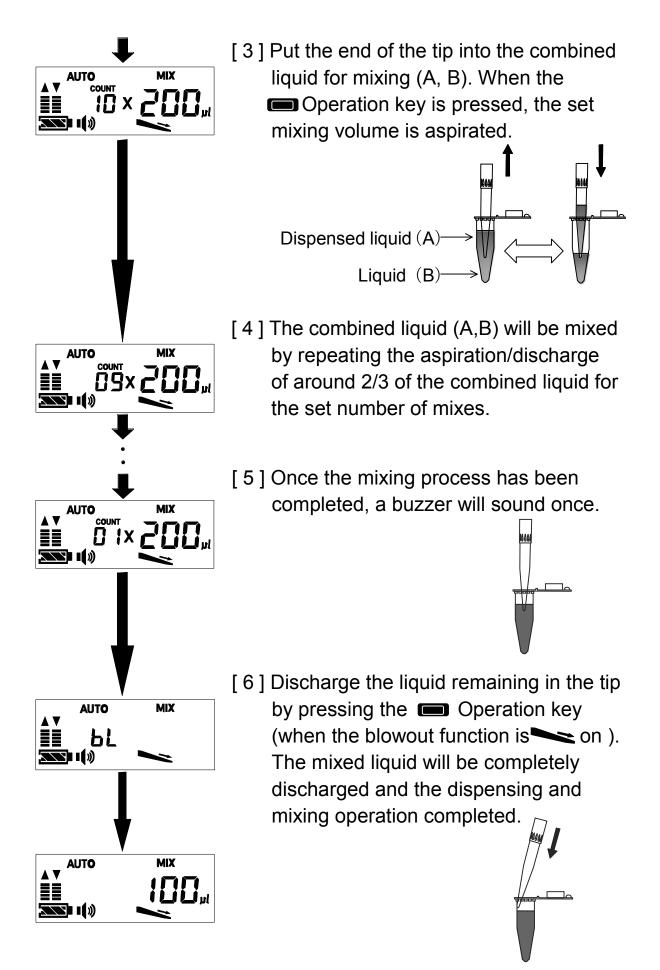
When the operation is complete, the buzzer will sound twice.
