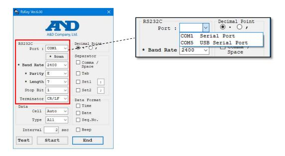
[Port:] Connect cable to appropriate COM port on the computer.
