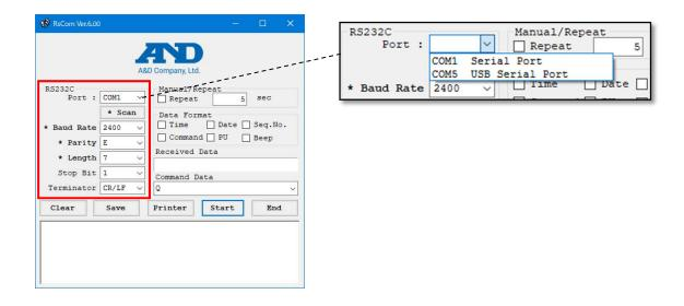
[Port:] COM port to which the cable is connected on the computer.
