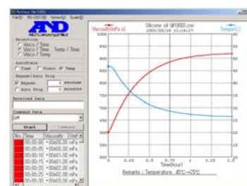
Figure 14 Real Time Display of Measured Data (WinCT-Viscosity)
