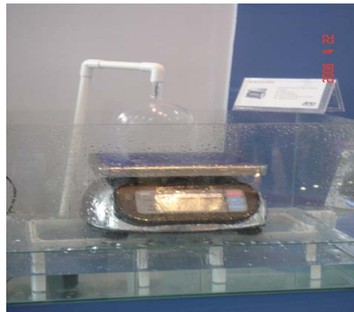
The waterproof and durable SK-5000WP being showered with water
