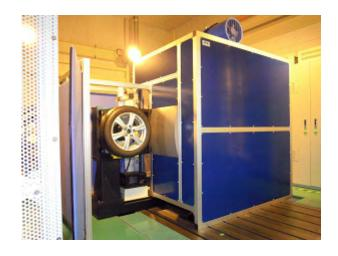
As these standards and regulations increase the demand for improved drivability, more realistic testing is required, including the introduction of flat-surface tire testing with a testing machine equipped with a steel belt.
