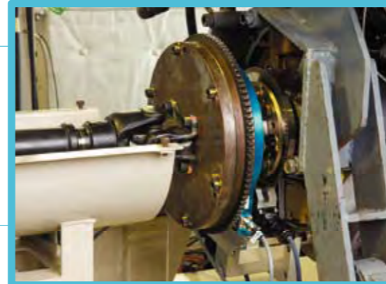
Operation example with direct coupling to an engine crankshaft at A&D's Engine Test Cell
