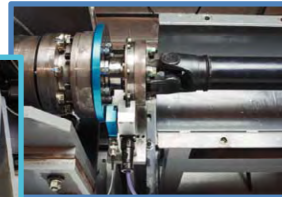
Installation example of coupling to dynamometer intermediate shaft at A&D's Engine Test Cell
