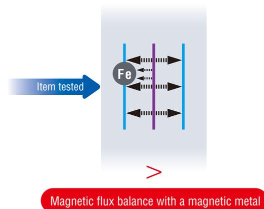
When a product contains a non-magnetic metal (stainless steel, SUS), magnetic flux to a receiver coil decrease due to occurrence of an eddy current and this makes the differential signal output negative.
