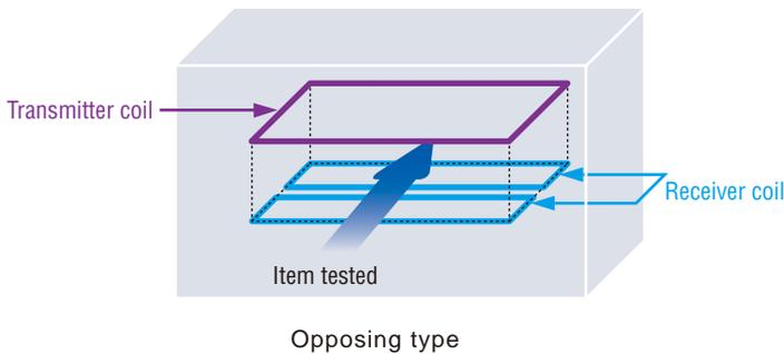
The opposing type metal detector allows for the manufacturing of a large size sensor head or for possible adjustment of the height of the aperture on request.
