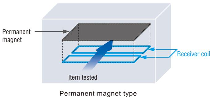
The permanent magnet type which can generate DC magnetic flux is used for detection of metal contaminants in aluminum foil packages.
