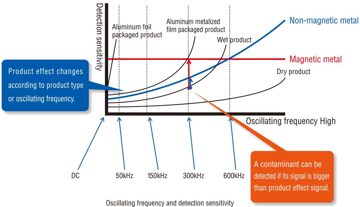
**Dry products :** The higher the oscillating frequency is, the better for detecting non-magnetic metals.
