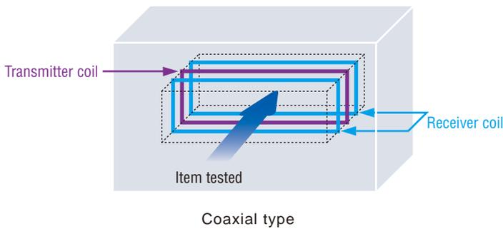
The AD4971 has adopted the coaxial type which is commonly used nowadays due to its high detection sensitivity and water resistance.
