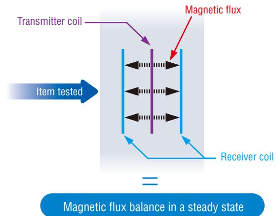
When an item contains magnetic metal (iron, Fe), magnetic flux to a receiver coil increase and this makes the differential signal output positive.
