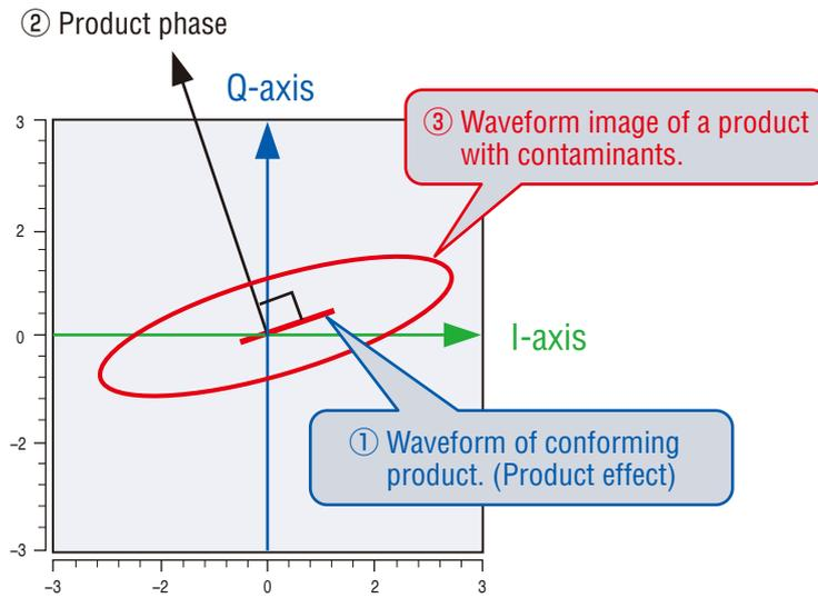
On the product effect graph, product phase is represented by the phase at the point of the V-shaped waveform.
