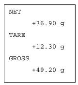
Example of output with GX-A/GF-A series multi-functional precision balances
