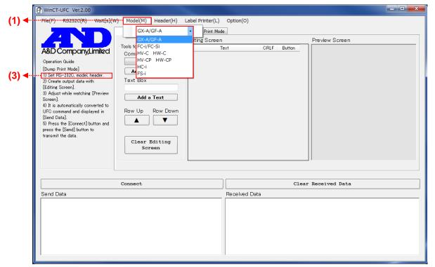
When the model is selected, the list of usable UFC command headers is shown in **Header(H)** (1). Choose one according to the intended application.
