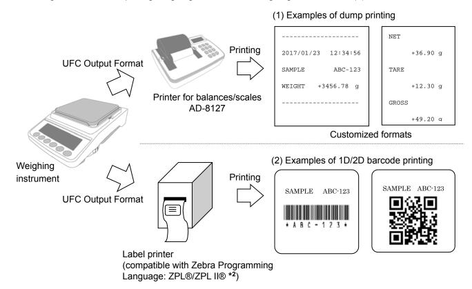
With UFC Output Format, the following three can be output: Static text, variable data that a weighing instrument holds (such as weighing data) and the control code in ASCII. Each of them can be combined with the others to be output together.
