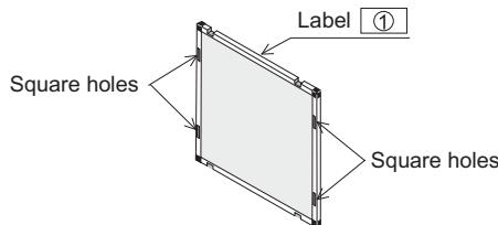
Step 2. Assemble the left side panel ② and the back panel ① using the hooks and the square holes.
