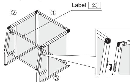
Step 4. Assemble the front beam panel ④ in the same way as steps 2 and 3.
