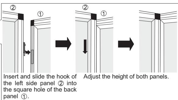
Insert and slide the hook of the left side panel ② into the square hole of the back panel ①.
