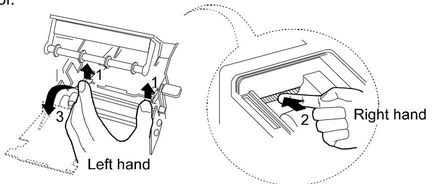
5. To reinstall the paper guide, slide it in until the rear end reaches the printer casing while taking care not to touch the paper sensor, then hook on the catch to secure the paper guide in place.
