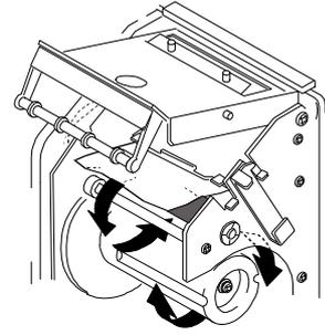
7. Secure the paper using the paper securing fixture. Pull the paper edge by hand so that no slack exists in the paper.
