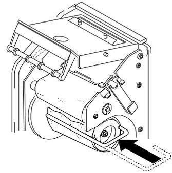
8. Secure the print head using the head securing fixture. If any labels remain near the print head, remove them.
