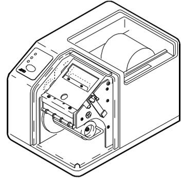
2. Release the head securing fixture to raise the print head.
