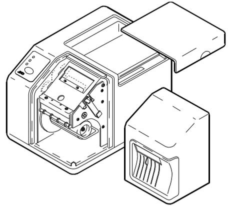
2. Release the head securing fixture to raise the print head.
