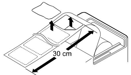
5. Remove the paper securing fixture from the paper take-up core.
