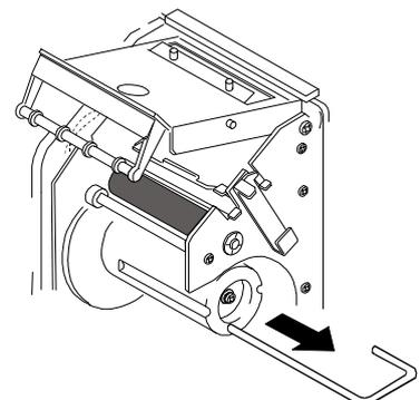
6. Thread the paper through the paper guide, fold the paper at the label peeling bar and place the paper on the paper take-up core.
