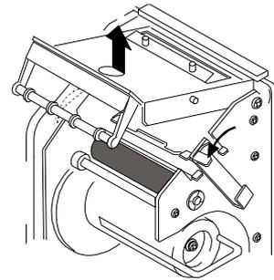
3. Raise both ends of the paper guide as shown below, release the catch, and push lightly from behind to slide the paper guide forward.
