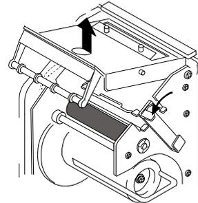
3. Attach the roll core to the paper. Place the paper in the paper holder as shown.
