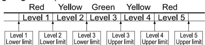
To use the comparator modes, the function settings “[P-L]” and “[P]” must be specified and the comparator values must be set.
