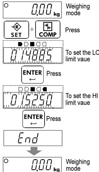
\* With the HV-C models, the scale changes the readability digit depending on the display range. Enter 0 for the final digit.
