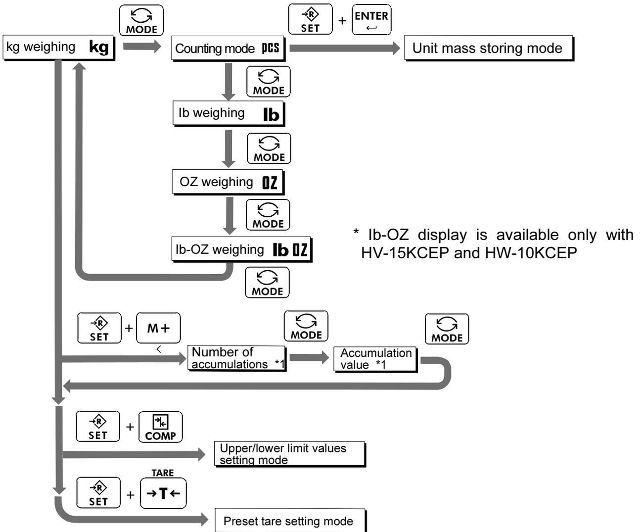
\* The scale displays the number of accumulations and an accumulation value only when accumulation data exists.
