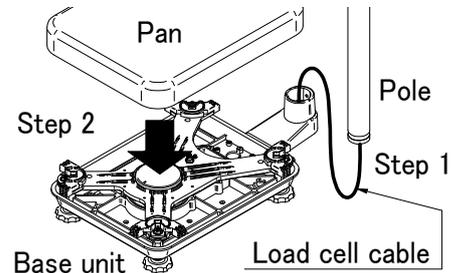
**Step 2** Place the pan on the base unit. Remove the protective film from the pan before use.
