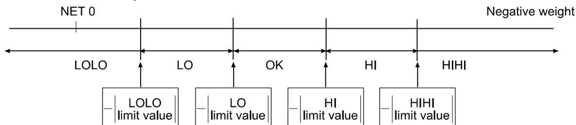
Note: To start the take-away check weighing, be sure to use the **[TARE]** key to tare the weight of the container filled with objects. The **[ZERO]** key may zero the display, and the scale goes below the zero point by taking out the objects. Then, the auto-tare function or **[TARE]** key does not work.
