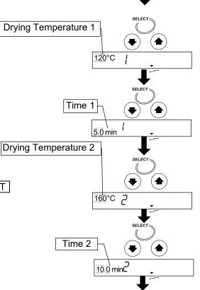
Note: Set "time 2" to the time from the start of measurement. (Refer to the list of Drying Program (Heating Pattern) on page 29.)
