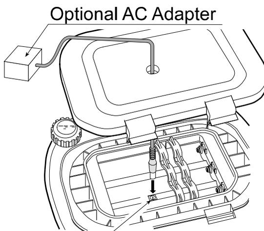
Plug the AC adapter to the AC adapter socket inside the battery compartment.
