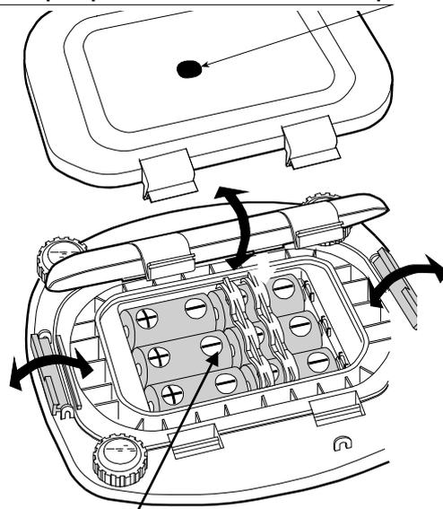
New six batteries. (R20P/ LR20/ D size)
