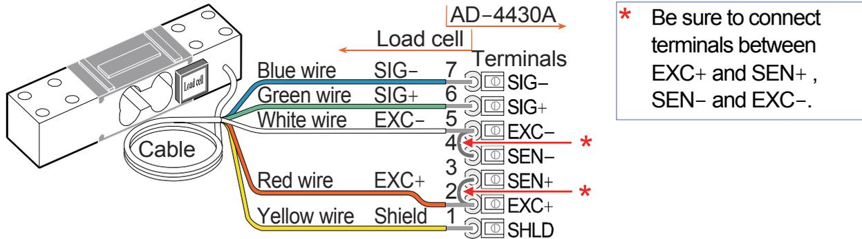
Illustration 6 Load cell connections (4-wire connection & direct connection)
