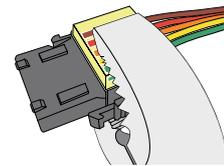
Step 3 Be sure the cover and the body are parallel to each other and there is no space between the body and the cover.
