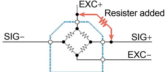
Illustration 11 Load cell output adjustment
