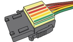
Step 2 Crimp the cover on the body using pliers from the side of the connector as shown in the illustration to the right.
