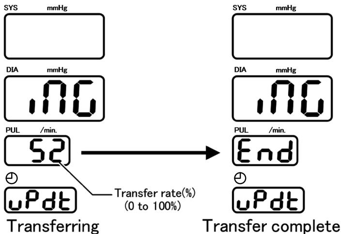
After transfer, restart the power, and then set the function **F15** to **2**. The bitmap is printed with the blood pressure value after blood pressure measurement.
