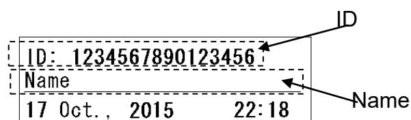
To input an ID, set the function **F20** to **3**, and connect an ID reader.
