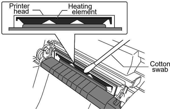
4. Clean the printer paper compartment to remove dust, paper debris and other foreign matter. Debris in the paper output path may lower the printing quality.
