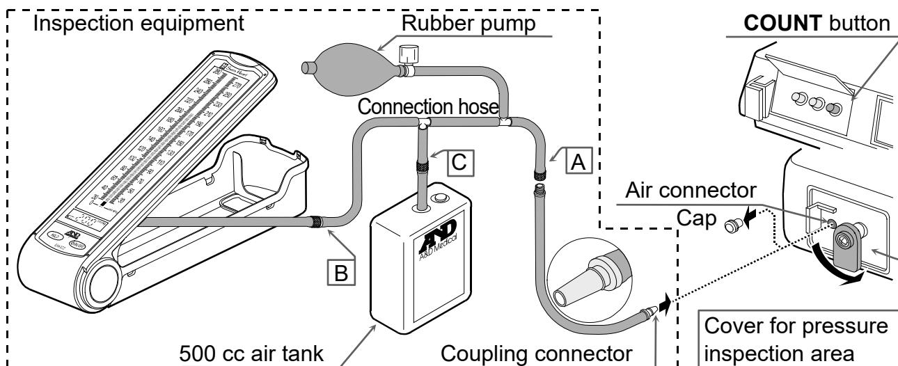
1. Hold the **COUNT** button on the rear of the blood pressure monitor, and turn the **POWER** switch on.
