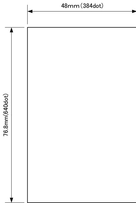
Create the bitmap data of the abovementioned size with a file name "Logo.bmp" and save it in the root folder of the SD card.
