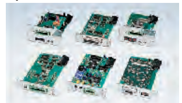
Top Row: DeviceNet, RS-232C and CC-Link Bottom Row: RS-422/485, Analog output, and PROFIBUS
