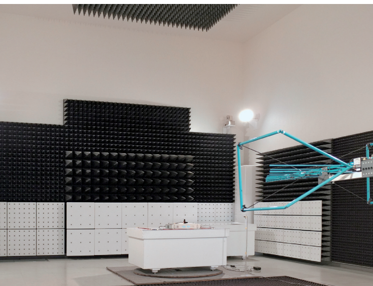
Anechoic chamber for EMC testing
