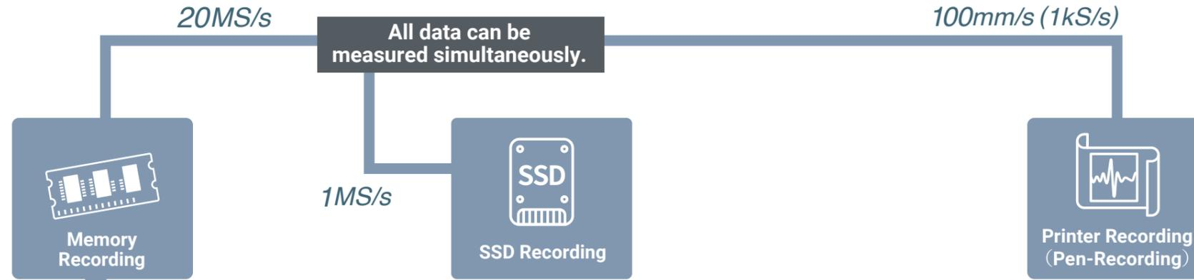
Memory mode records data in the internal memory (4GB) at high speed (Max: 20MS/s). In addition, measurement can be performed under a variety of conditions using a variety of trigger functions.
