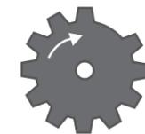
The gear to the left has 11 teeth, so the number of pulses per revolution is 11.
