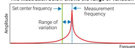
This module detects the frequency from the input pulse and calculates the variation from the set center frequency value. Changes in range of variation can be measured as sequential data.
