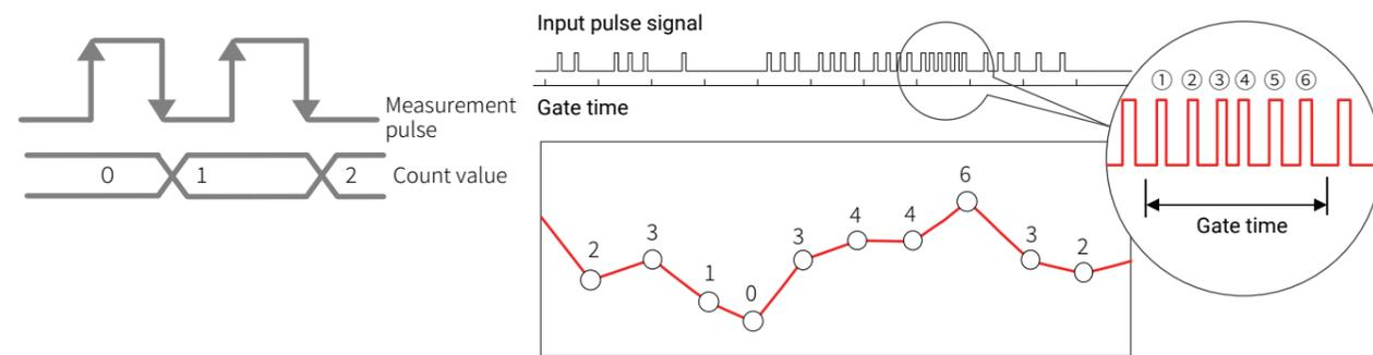
The number of pulse signals input within the gate time is counted and recorded.
