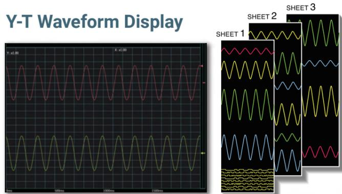
Display the measurement channels split into three sheets. Up to 48 channels of signals can be monitored on a sheet with 20 vertical/horizontal divisions. Graphs can be divided into 1 to 18 sheets and displayed.
