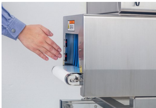
Safety sensors are embedded at access points to provide additional safety.
