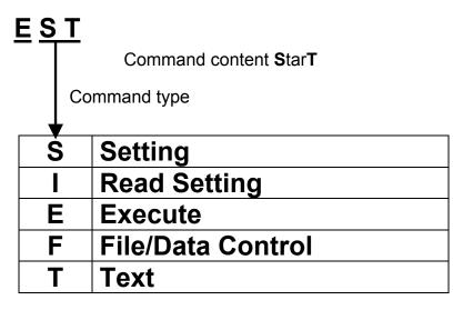
Input a parameter following the 3-character command. Insert a separator (comma "," or space " ") between parameters. When it is possible to omit parameters, it is necessary to insert commas in sequence instead of parameters in order to clearly indicate that the parameters are omitted. Lastly input a delimiter and operation is complete. Available delimiter s are [CR+LF], [CR], [LF] and it is necessary to use the same delimiter as that set in the RM1100.
