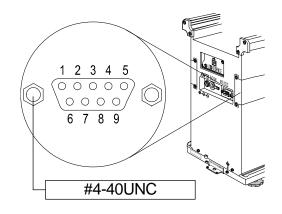
Signal names other than TXD and RXD are DTE-side names.
