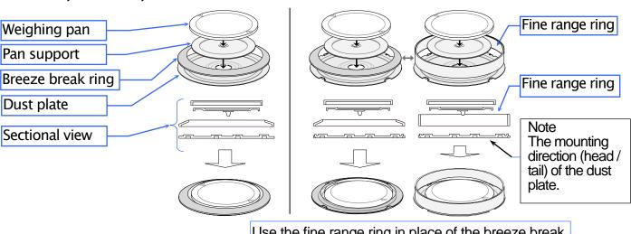
Use the fine range ring in place of the breeze break ring to avoid errors caused by drafts when weighing with a readability of 0.01 mg.
