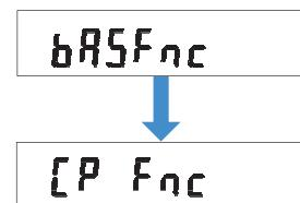
Step 2 Press the **SAMPLE** key to display **[P Func]** (Comparator).
