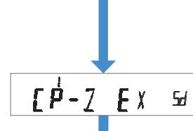
Step 6 Press the **RE-ZERO** key to display **[P-E] 1** (5-stage comparison).
