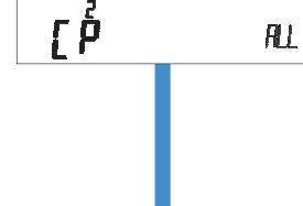
Step 4 Press the **RE-ZERO** key several times to display **[P] 2** (Comparison always).
