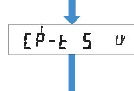
Step 5 Press the **SAMPLE** key to display **[P-E]** (Comparison method).
