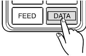
Whether or not to print data is selected alternately each time the DATA key is pressed in MODE 3.
