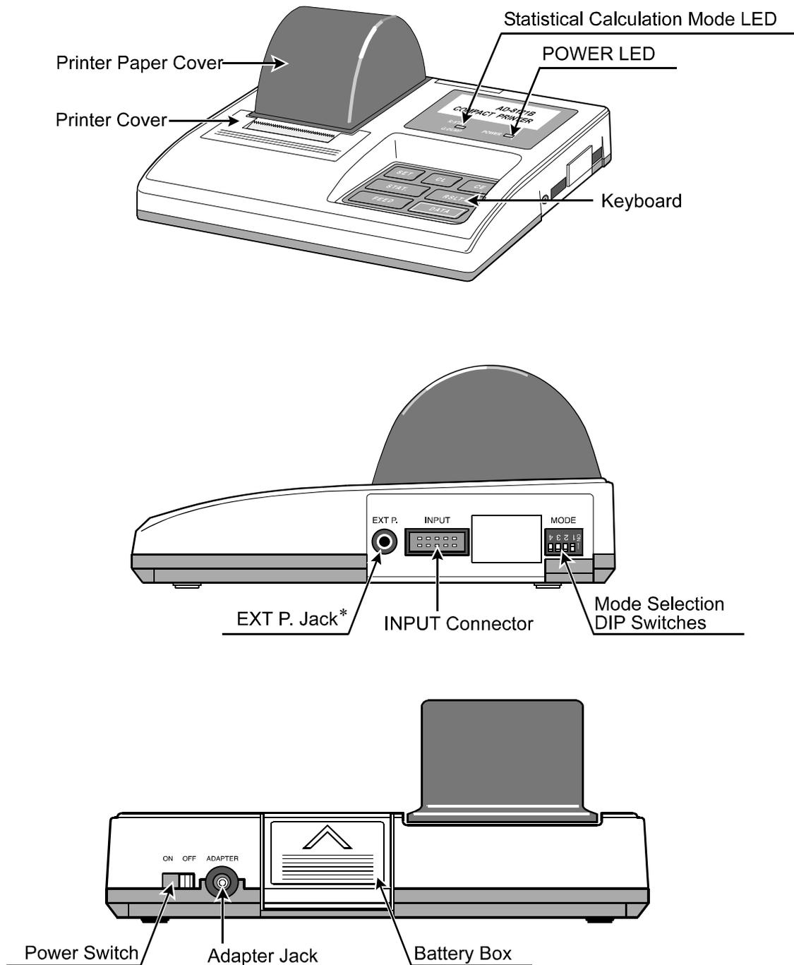
\* For data acquisition by pressing the foot switch, connect the plug to the foot switch, and then insert the plug into the EXT P. jack. The foot switch will function in the same way as the DATA key on the printer keyboard.
