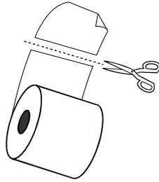
Step 4 Turn on the power. Press the FEED key while lightly feeding the printer paper edge into the paper inlet until it comes out of the outlet an appropriate length. Insert the supplied roller shaft into the printer paper core, then set the shaft onto the bearings of the printer.
