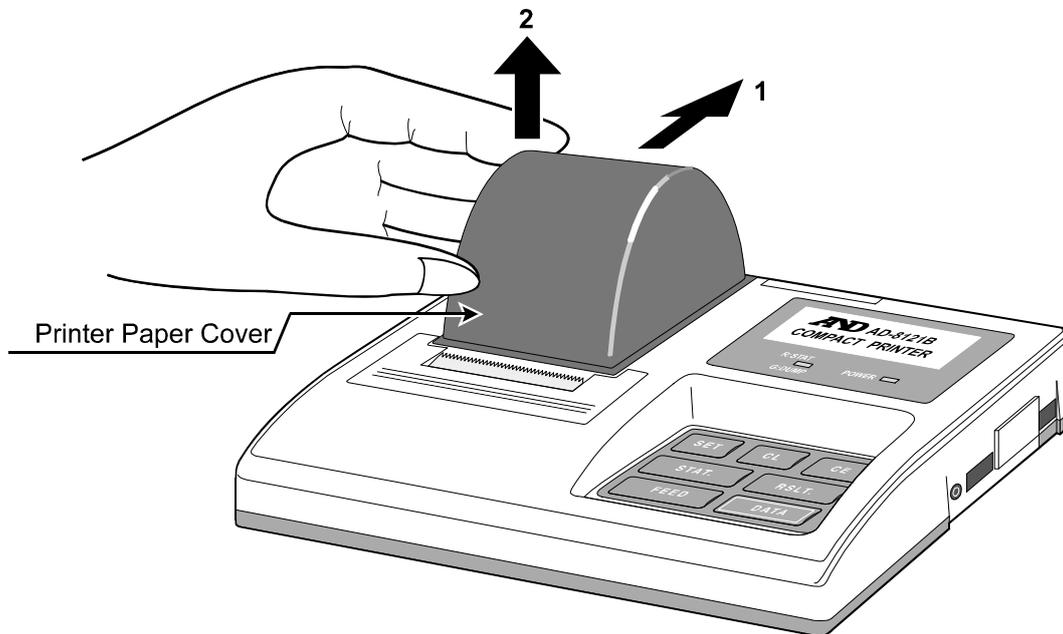
Step 2. Push the printer cover at the spot marked by the arrow (1). Remove the printer cover (2).
