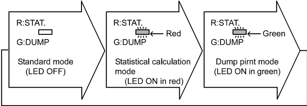
When the date is set to be printed, the date will be printed when the printer is set from the standard mode to the statistical calculation mode.
