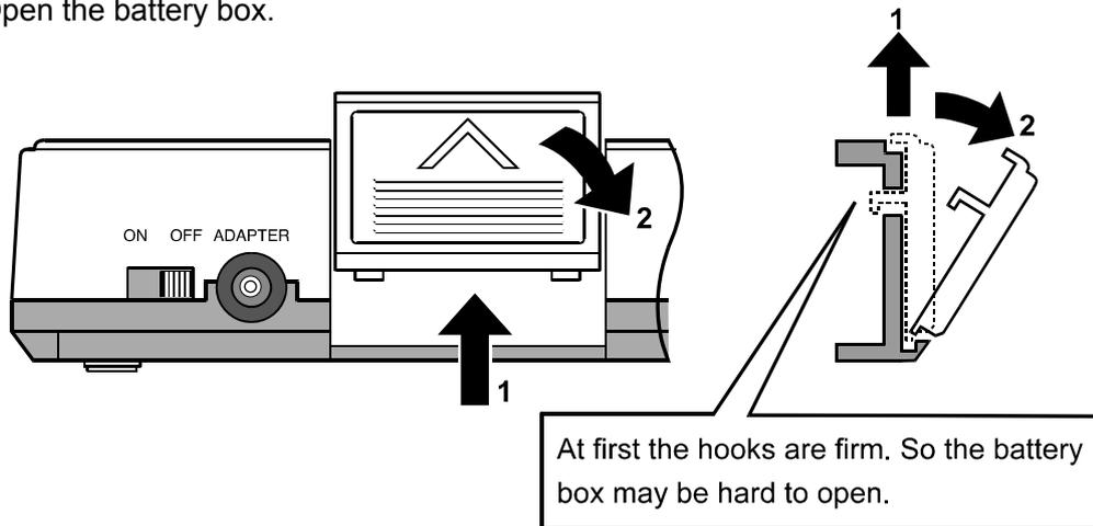
Step 2. Install the batteries.
