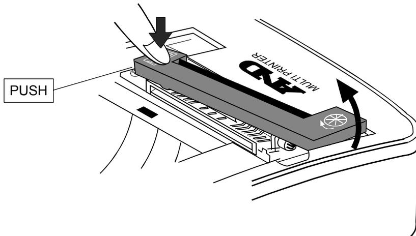
3. When attaching the ink ribbon, turn the ink ribbon's knob in the direction indicated by the arrow until there is no slack in the ribbon.
