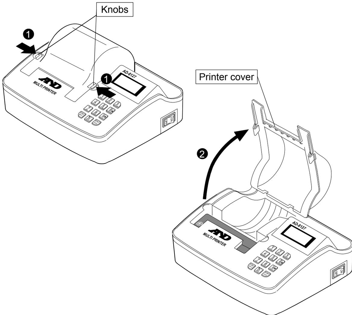
**Note** Opening or closing the printer cover improperly may result in damage to the printer cover.
