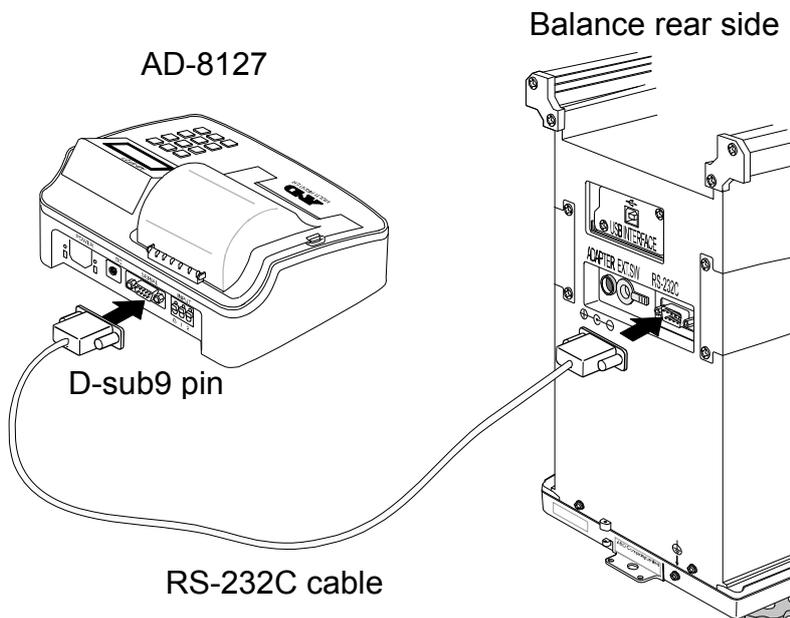
\* Depending on the balance or scale models, there are three types of pin: D-sub9 pin, D-sub25 pin or Din7 pin. Use the cable that matches the specific type to connect the printer.
