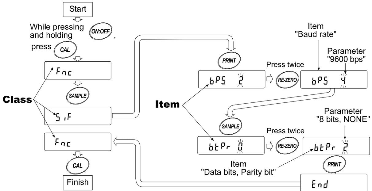
**Note:** Use much care when changing parameters. The AD-8922 may not function properly when the settings and operational environment are not appropriate.
