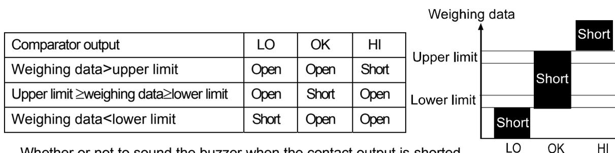
Whether or not to sound the buzzer when the contact output is shorted can be set in the "Buzzer mode ( $bEP$ )" of the "Comparator ( $[P Fnc]$ )".
