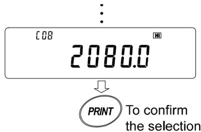
**Note:**                      When no operation is performed in step 4 (after a few seconds of inactivity), the AD-8922 selects the value currently displayed and returns to the weighing data display automatically.
