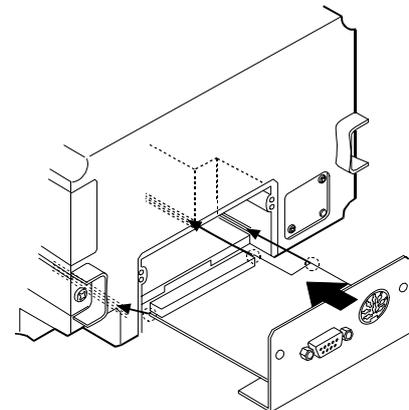
4. Using the two screws removed in step 2, fasten the option board.
