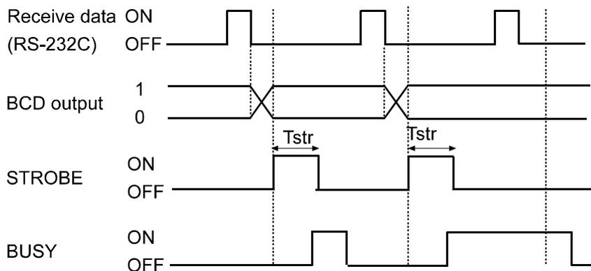
“BUSY input ON” is the condition that BUSY is connected to input signal GND (Pin 3).
