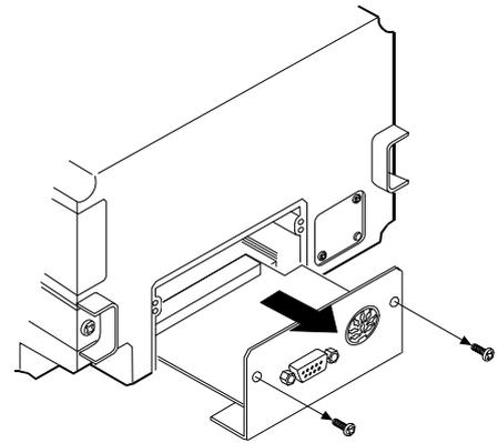
3. Insert the option board, along the guides on the left and right sides.
