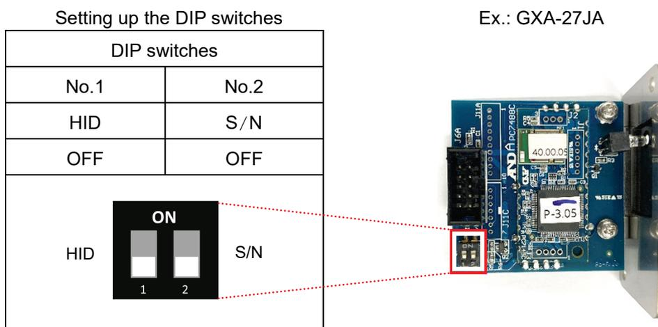
4. Attach the option board to the weighing device again, as indicated in the instruction manual of the option board.
