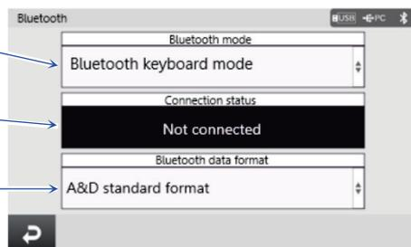
2. Set the Bluetooth mode to Bluetooth serial, and the Data format to A&D standard format.
