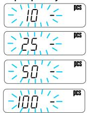
When the sample weight is light and the counting error could become large, the balance will request you to use larger number of samples.
