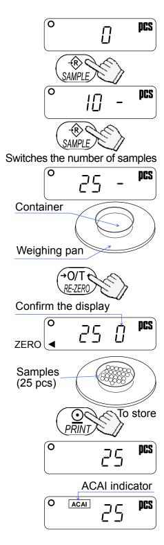
10. Counting accuracy is improved when the ACAI indicator turns off. Each time the above operation is performed, a more accurate unit weight will be obtained. There is no definite upper limit of ACAI range for the number of samples exceeding 100. Try to add a similar number of samples as that displayed.
