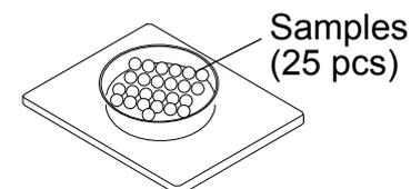
6. Press the **ENTER** key to calculate and store the unit weight. Remove the sample. The balance has been set to count objects with this sample unit weight.
