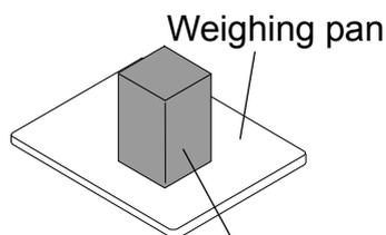
5. Press the **ENTER** key to store the 100% reference weight. Remove the sample.
