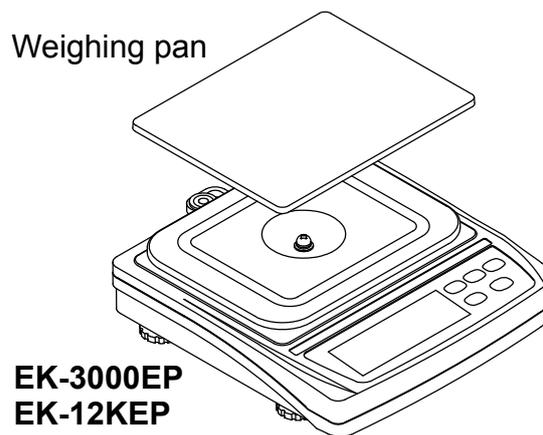
2. Place the balance on a solid and level surface. Adjust the level of the balance using the leveling feet. Use the spirit level to confirm. The bubble should be in the center of the circle.
