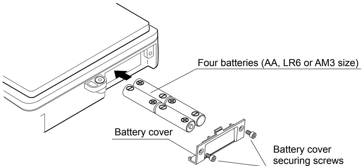
4. Attach the battery cover and secure it to the balance using the battery cover securing screws.
