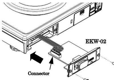
Step3 Secure the EKW-02 with the screws supplied with the EKW-02.
