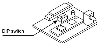
Note: To switch the DIP switch settings, use a rounded object such as the tip of a ballpoint pen to slide it.
