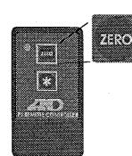
Use the ZERO button to move the flashing digit to the one you wish to change.
