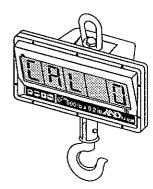
Ensure no weight is on the hook - no chains, slings etc.
