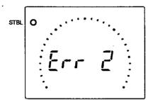
Err 2 is displayed if there has been a failure in the non volatile RAM.
