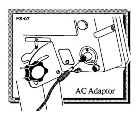
Insert the adaptor lead into the grommet and push it firmly home into the socket.
