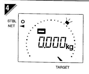
Press the TARE key to zero the weight display and light the NET annunciator.
