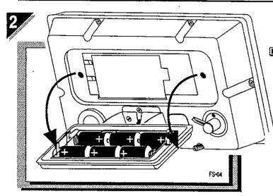
Carefully fit the 6 x C cells into the carrier observing the correct polarity as marked inside the battery cover.
