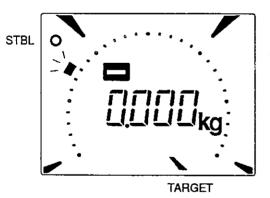
O The TARGET annunciator will come on and the analog part of the display will flash at the previously set TARGET weight.
