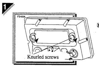
Remove the battery compartment cover by undoing the 2 knurled securing screws and pulling the cover away from the rear of the display.
