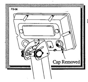
Remove the cap, on it's retaining strap, from the end of the adaptor inlet grommet.
