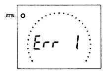
Err 1 is displayed if there was a weight on the pan when the scale was switched ON.
