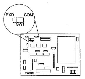
O Position **COM** if you are to use the comparator output relays
