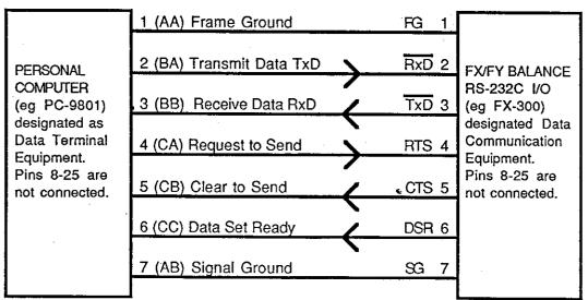
\* Use a high quality modem type cable between the computer and balance.
