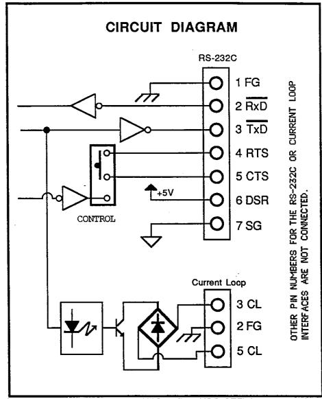
A 25-pin RS-232C male connector and cover (HDB-25P & HDB-CTF) is not provided with this option. A 7-pin DIN male Current Loop connector (TCP 0576) is provided for the passive Current Loop interface. The CONTROL switch on the PCB permits shorting RTS and CTS lines, or for the balance to send the Clear to Send signal (RTS and CTS are normally shorted).
