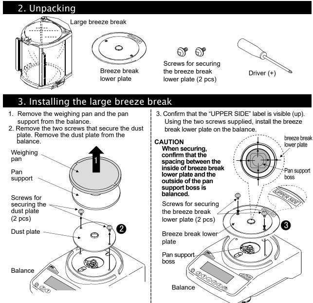
CAUTION - When installing, use care not to apply excessive load to the sensor mechanism (circumference of the pan support boss) of the balance.
