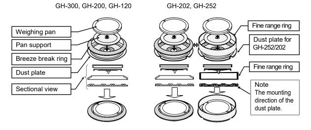
Use the fine range ring in place of the breeze break ring to avoid errors caused by drafts when weighing with a readability of 0.01 mg.
