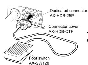
The external input connector (AX-HDB-25P/CTF) and the foot switch (AX-SW128) are sold separately.
