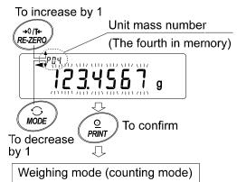
3 Press the PRINT key to confirm the selection and to return to the weighing mode. To cancel the selection and return to the weighing mode, press the CAL key.
