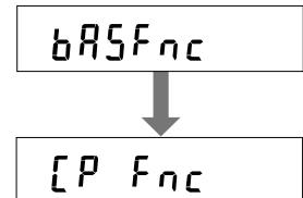
Step 2 Press the **SAMPLE** key to display **[P FnC]** (Comparator).
