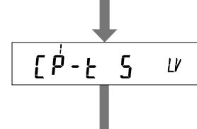
Step 5 Press the **SAMPLE** key to display **[P - t]** (Comparison method).
