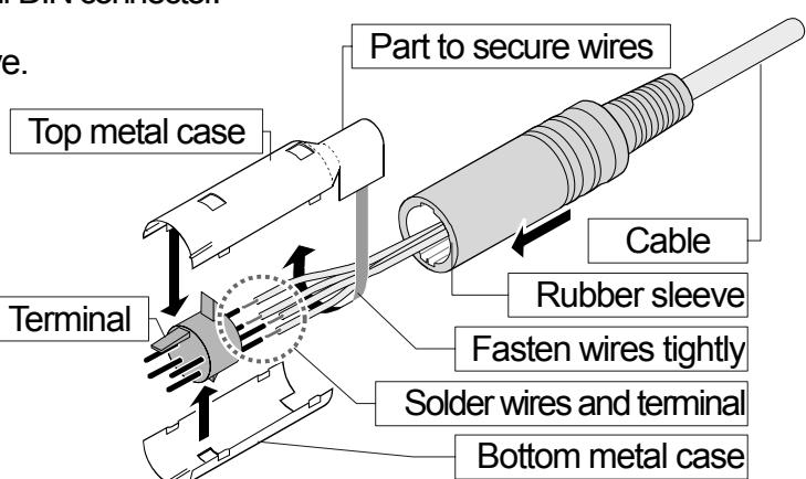
Step 2 Solder wires and terminal.
