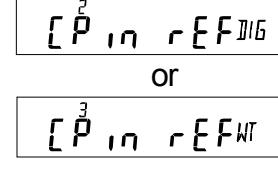
Step 8 Press the **RE-ZERO** key several times to display **[P - I] 1** (Comparison excluding  $\pm 5$  digits (counts) from zero).
