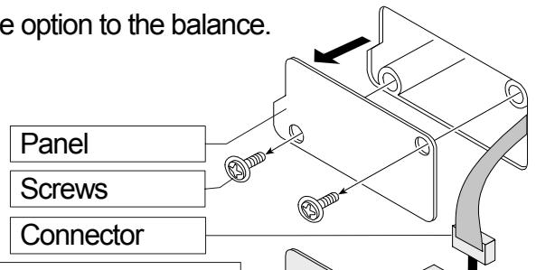
Step2 Peel off the connector that is affixed to the panel with double-sided tape and insert it into the socket of the option board.
