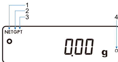
Indicators for the net / gross / tare function in use
