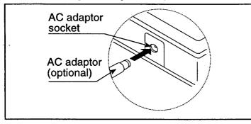
Plug the AC adaptor to the AC adaptor socket on the side.
