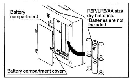
Remove the battery compartment cover and insert six batteries (R6P/LR6/AA size) into the battery compartment, taking extreme care that the polarities plus and minus are observed.
