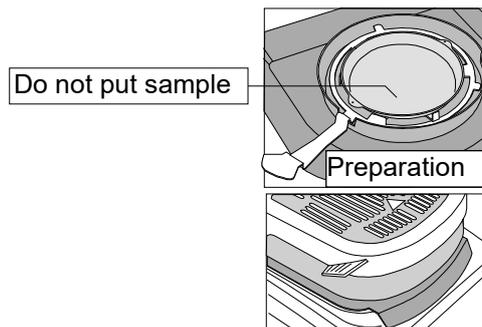
If **[CLOSE]** is displayed, the heater cover is not closed. When it is closed, the self-check function is started.
