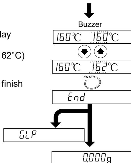
When the heater cover is opened during measurement or the STOP key is pressed, calibration is stopped and the analyzer displays the weighing mode.
