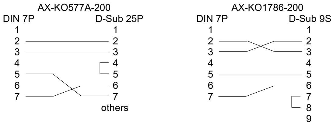
(DIN 7 pin plug P can connect with DIN 8 pin socket.)
