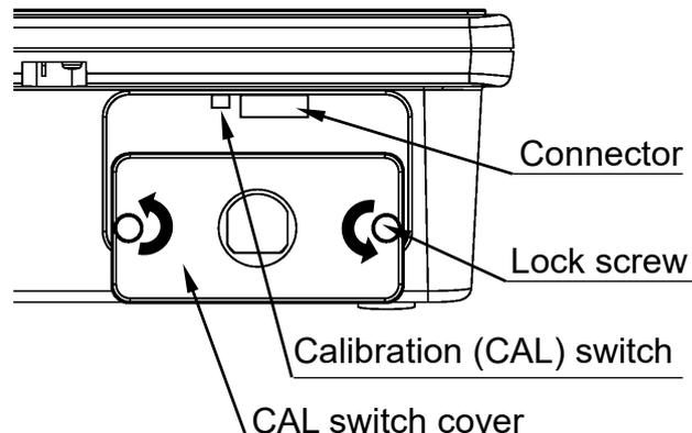
Loose the lock screws on the rear side of the display pod, and remove the CAL switch cover. Then, there is a calibration switch on the board inside.
