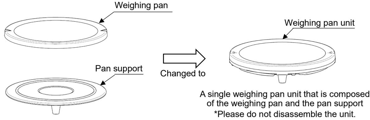
Weighing pan and pan support (separate components)
